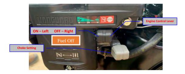
4. Moving the Top Black lever to the Right – Stops the engine from running and Shuts off the Fuel Valve. Move to the Left to Run.
